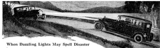
This picture illustrates the danger of up-tilted headlights in blinding the other fellow on the road. The dazzling effect is increased when the car is going over the brow of a hill
